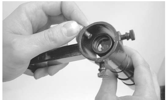
Figure 3. Pull the spring-loaded tensioner outward, then insert the finder scope into the finder scope bracket.
