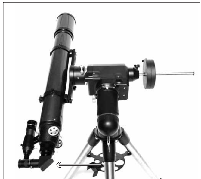
Figure 7. Gently push the telescope horizontally to determine the direction of optical axis offset.
